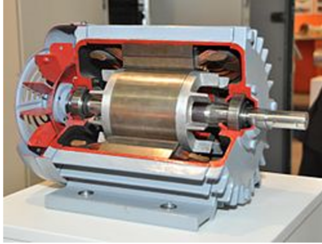
Figure 20: Principle of Induction Motors
